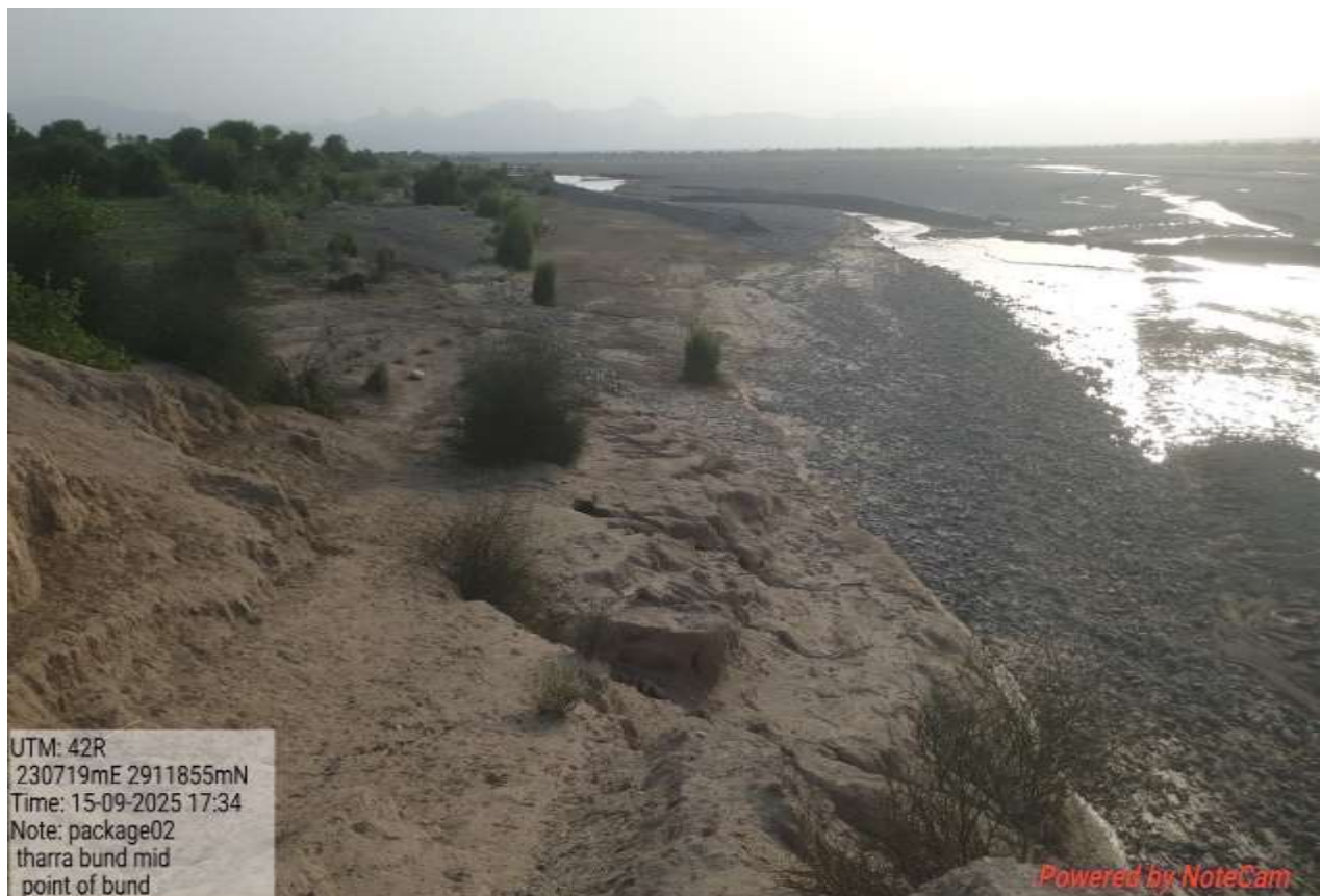
Figure-3-3: Alluvial deposits (Clayey Silt, Silty Clay and Gravely Silt) along the riverbank.
