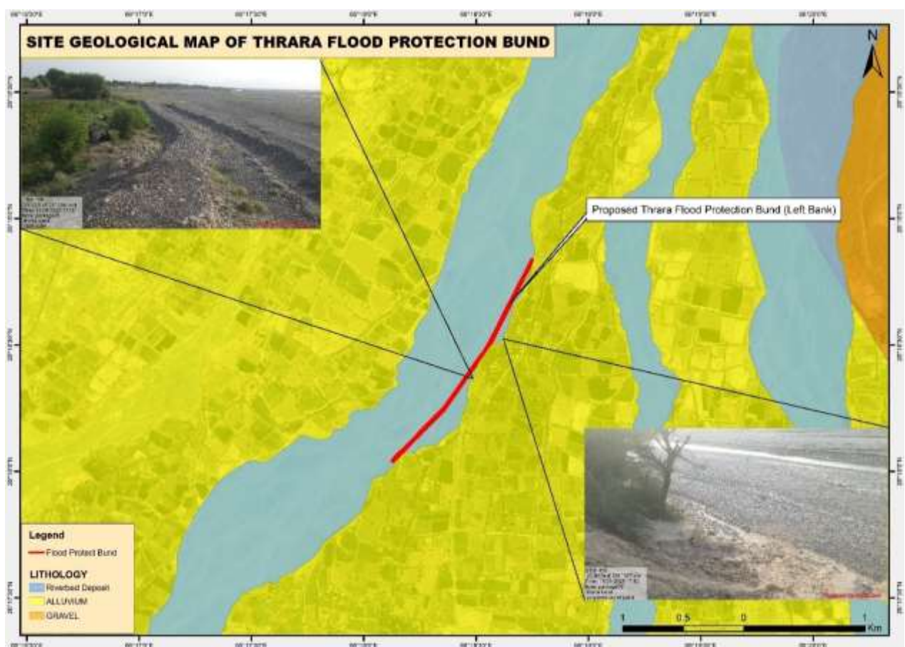
Figure-3-4: Surface geological map of the Thrara flood protection bund.
